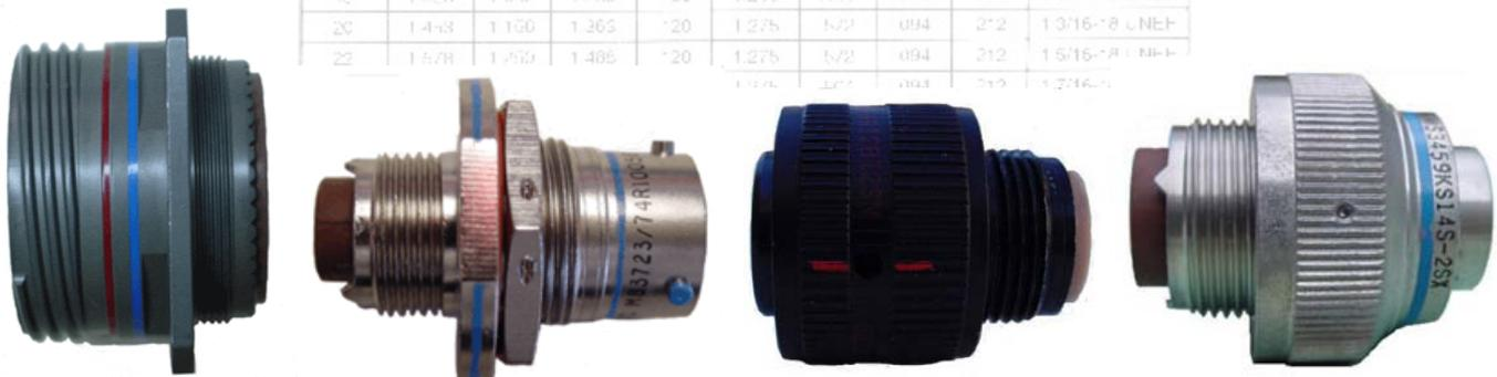
Finish is next and just as important as shell size. Finishes come in a wide variety to fit the most diverse connector requirements from olive drab over cadmium to electroless nickel aluminum to black anodized to stainless steel as shown above from left to right. If the finish is part of the environmental class for the connector family, you have already done this.
